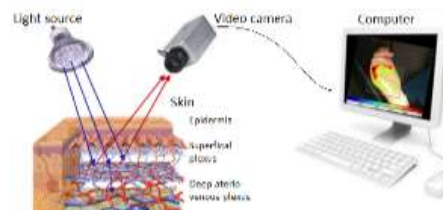
Fig. 1 The principle of rPPG technique.
